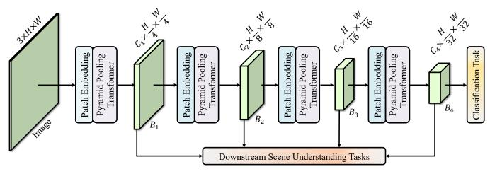
Fig. 2. Architecture of the proposed P2T network. We replace the traditional MHSA with our pooling-based MHSA. The feature maps  $\{B_1, B_2, B_3, B_4\}$  can be used for downstream scene understanding tasks.
